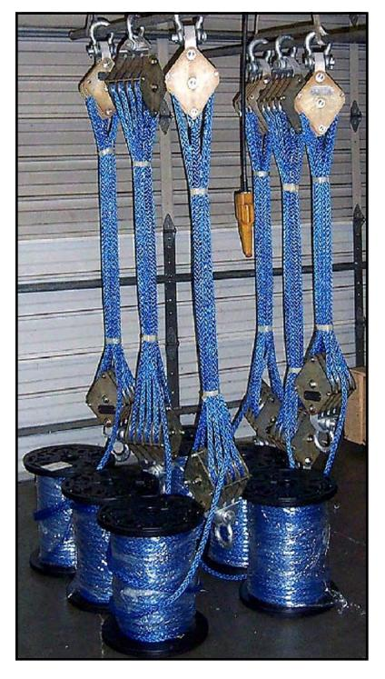
8 Part block and tackle ready for use. This set of block and tackle has been specifically designed for the line stringing industry with a robust, simple design.
