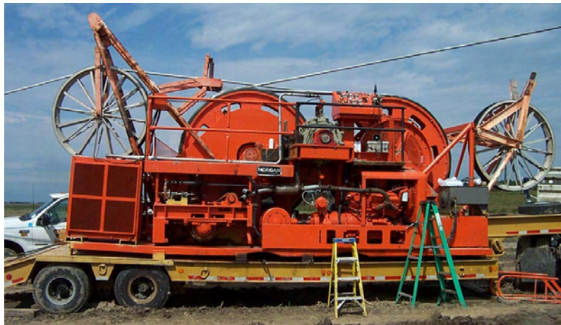
LH41-96-1 (96" dia bullwheels, single) River Crossing Tensioner
